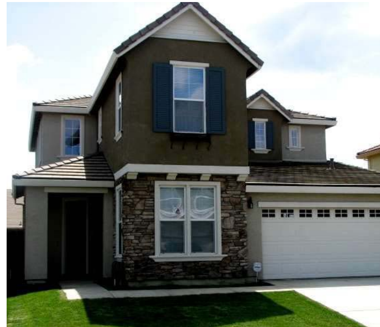
The height, mass, and appearance of residential homes should include some variation. Use texture and color to vary the articulation of the lower floor of a two-story house.
