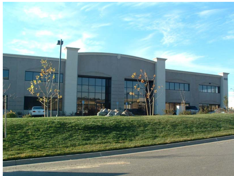
Screen parking from view of public street with the use of landscaped berms..
