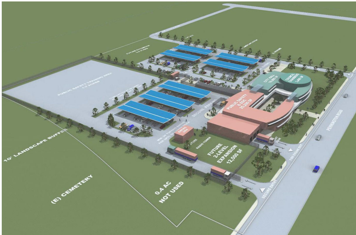
Figure 2 – Site A: Civic Center at Build-out with Photovoltaic (PV) System on Carports
