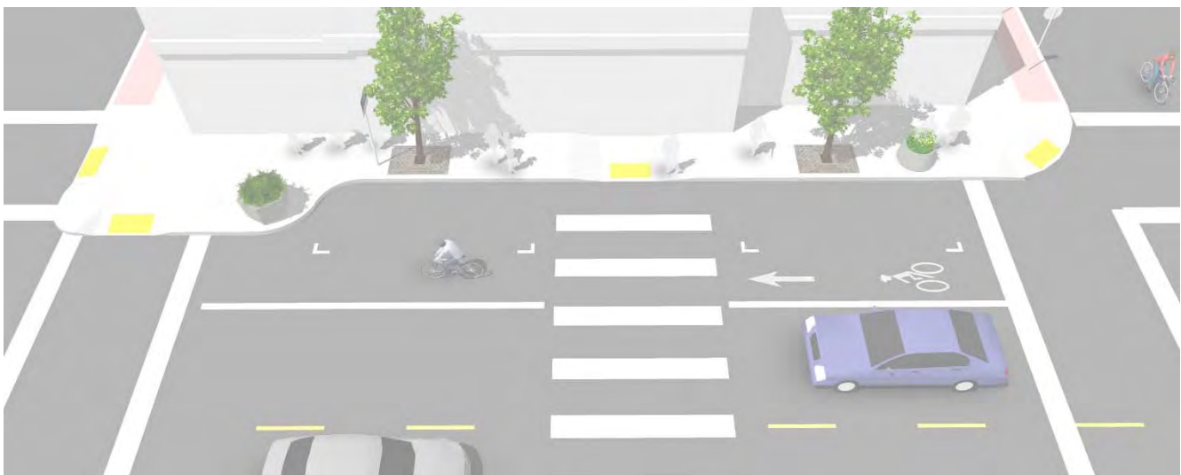
Perpendicular Curb Ramps
