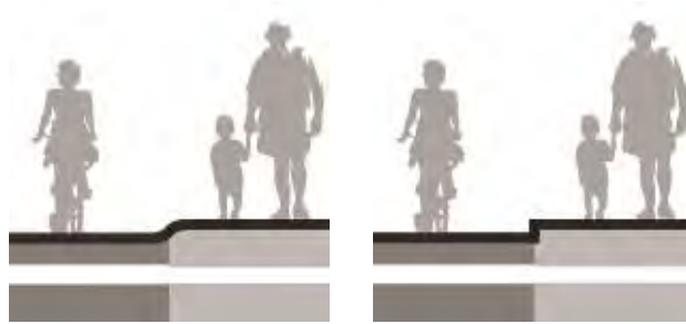
Rolled Curb vs Vertical Curb
