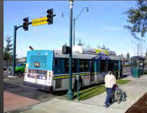
Separated sidewalk with narrow grass strip next to travel lane.
